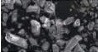
Conventional sodium bicarbonate powder Average particle diameter : 73 µm Scanning electron microscope image magnification of 150x
