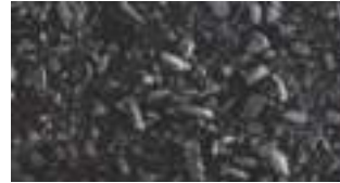
Perio-Mate Powder (glycine) Average particle diameter : 25 µm Scanning electron microscope image magnification of 150x
