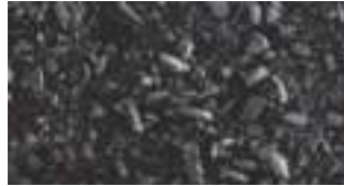
FLASH pearl (calcium carbonate) Average particle diameter : 54 µm Scanning electron microscope image magnification of 150x
